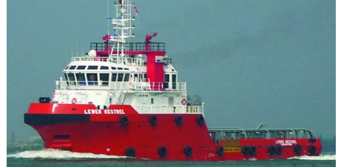
Hull #4878 2007 157' Anchor Handling Tug Lloyds+100A1 Tug Fire Firting Ship + LMC Unrestricted Service
